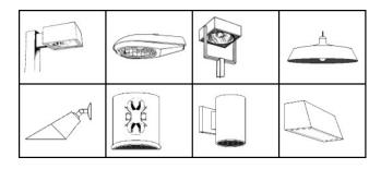
\*Note: To be fully shielded these fixtures must be closed on top and mounted such that the bottom opening is horizontal.
