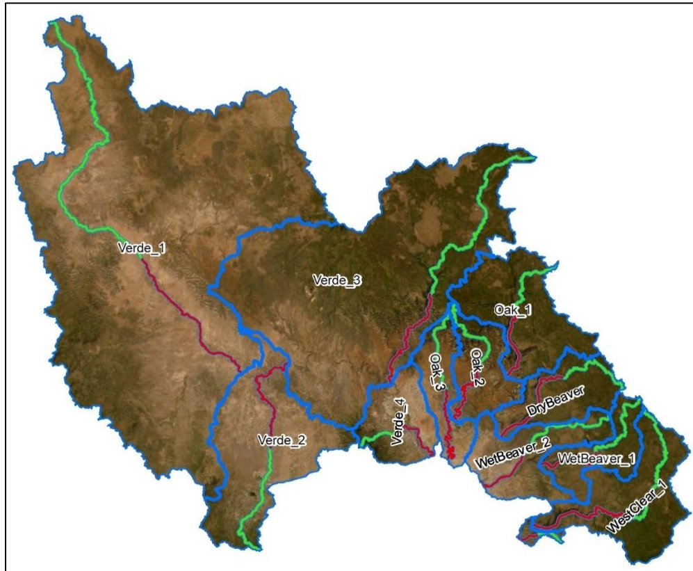
Figure 4-7. Longest Flow Paths (L, in green) and Length from Centroid (Lca, in red)
