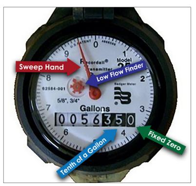
"Sweep Hand" records every 10 gallons used. The small six pointed red star or triangle is called a "Low flow finder" or "Leak detector". It will move if you have even a very small leak. Sometimes the movement is jerky and you might have to watch it for a few minutes.
